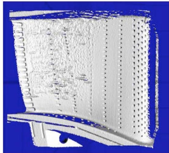
**Fig.6: Rendered laser scan of a volcanic ash damaged HPT NGV (Bonilla [2012]); this “discrete” geometry is available as a (tessellated) Point Cloud**
