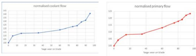
**Fig.24: Predicted variation in cooling flow & primary flow during the simulated “burn-through”**
