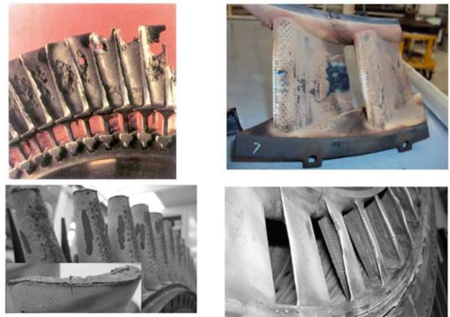
**Fig.3: Typical in-service degradation: (top left) hot corrosion (Wing *at al* [1981]), (top right) deposition & erosion on a HPT NGV (Batalha [2012]), (bottom left) HPT blade deterioration pattern & (bottom right) HPT vane damage – Trailing Edge bulging (both from Ebmeyer *et al* [2011])**
