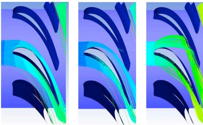
**Fig.13: Predicted trajectories of different sizes of particle: (left) 2  $\mu\text{m}$ ; (centre) 20  $\mu\text{m}$ ; (right) 200  $\mu\text{m}$**
