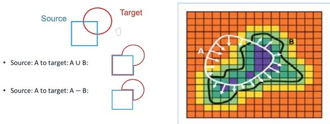
**Fig.8: Digital Geometry editing the Distance Field: (left) simple Boolean operations; (right) morphing Shape “A” to Shape “B”**
