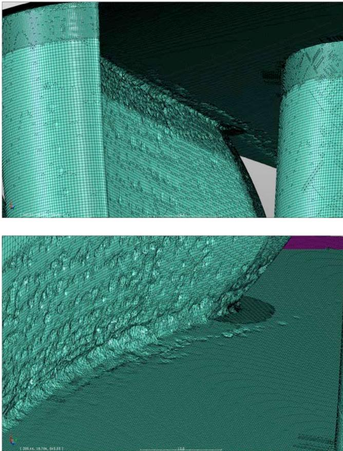
**Fig.16: Simulation mesh (surface shown) for the eroded stator blade; particularly evident is the erosion pattern associated with the particulate vortical structure formed in the pressure side/endwall corner.**
