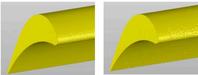
**Fig.18: The Level Set geometry can be morphed to interpolate between the pristine & eroded geometry and controlled by a “slider”:**
