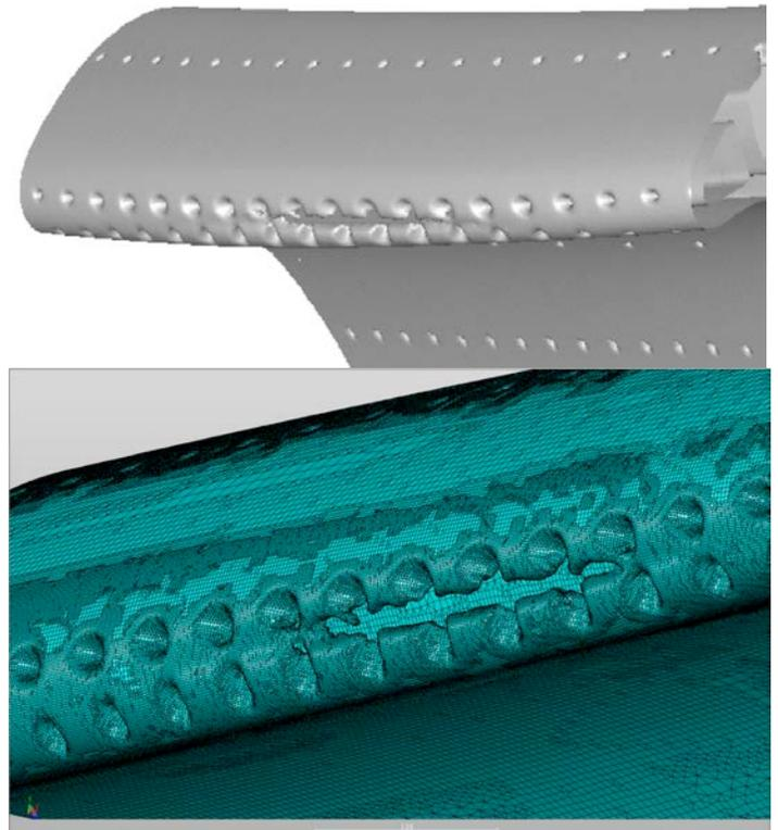
**Fig.22: Geometry (top); the zero distance of the Digital Geometry Level Set and associated mesh (bottom) in the later stages of the burn-through simulation.**
