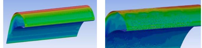
**Fig.20: Predicted flowfield (pressure) in the leading edge region of the pristine (left) & eroded (right) blades**
