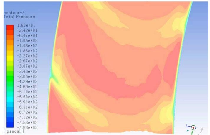
**Fig.17: Predicted total pressures near the vane TE for the pristine (top) and eroded (bottom) geometries.**
