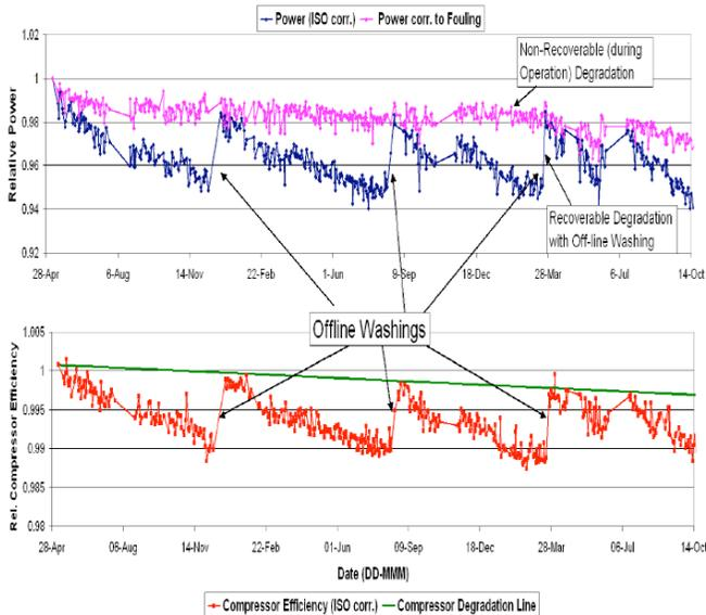
**Fig.1: The impact of compressor fouling & washing on engine performance (from Kurz *et al* [2014])**
