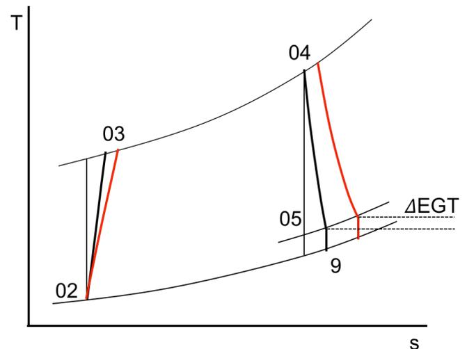
**Fig.5: Classic thermodynamic cycle for the core of a by-pass turbofan engine showing the effect of component degradation on efficiency (black to red)**
