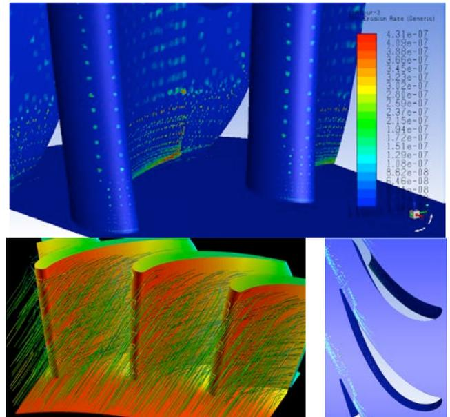
**Fig.14: Overview of predicted erosion rates in  $\text{kg/m}^2 \text{s}$  for the HPT stator vane**
