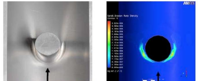
**Fig.12: Measured erosion (left) by sand particles of an aluminium cylinder/endwall compared with a Fluent™ simulation (right; taken from Graham *et al* [2009])**
