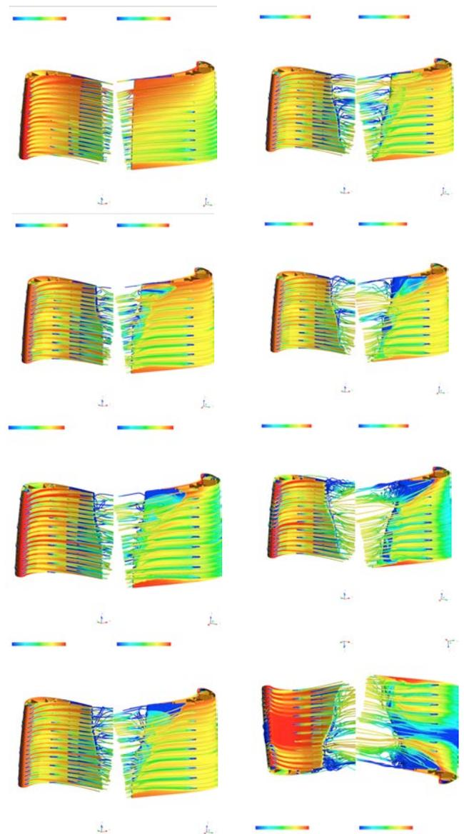
**Fig.23: Stages during the simulated “burn-through” of the cooled turbine blade: *flow simulation***
