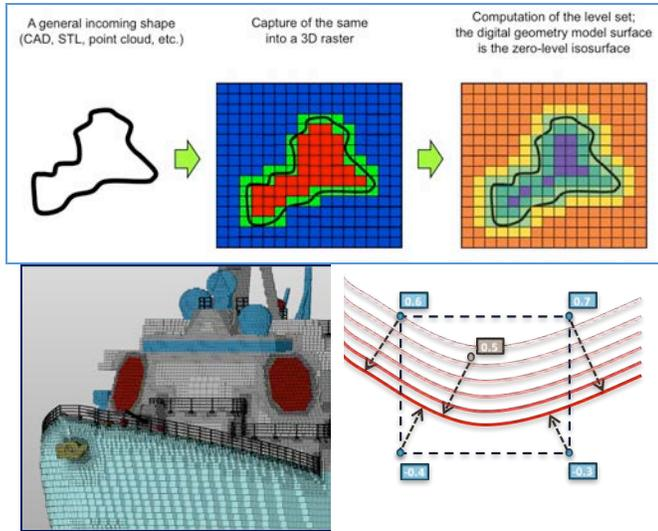
**Fig.7: Our Digital Geometry Kernel; on the (top) the “Rasterisation” of the geometry; on the (lower left) a 3D voxel image; on the (lower right) the Level Set Distance Field storing sub-voxel scale geometry information**
