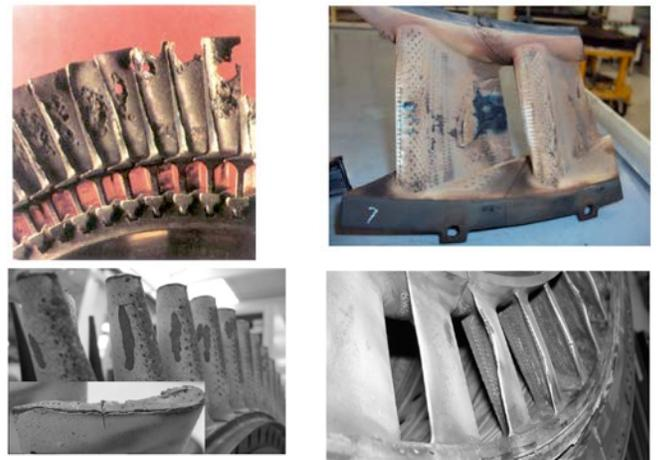
**Fig.3: Typical in-service degradation: (top left) hot corrosion (Wing *at al* [1981]), (top right) deposition & erosion on a HPT NGV (Batalha [2012]), (bottom left) HPT blade deterioration pattern & (bottom right) HPT vane damage – Trailing Edge “bulging” (both from Ebmeier *et al* [2011])**
