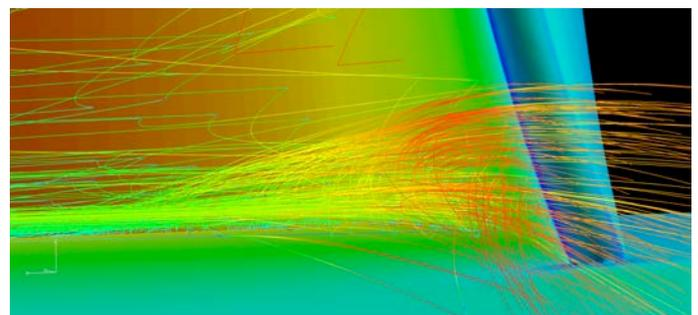
**Fig.15: Particle trajectories in the pressure side/endwall corner showing a vortical structure (view upstream from the blade trailing edge)**
