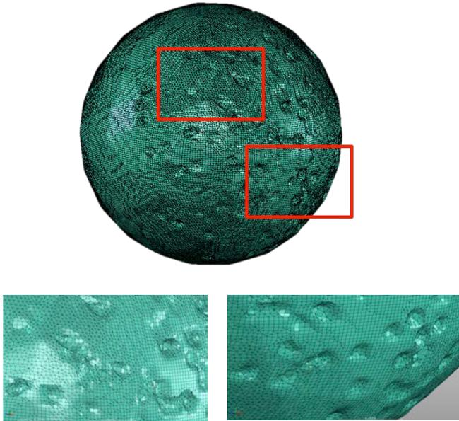
**Fig.10: Simulation mesh (surface shown) generated by our simulation system for the eroded sphere generated from the morphed Level Set geometry**
