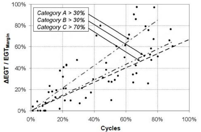
**Fig.2: The reduction of EGT margin with engine flight cycles for different airport environments A, B & C; Category A suffers mainly dust & sand erosive damage (from Ebmeyer *et al* [2011])**
