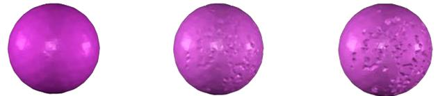
**Fig.9: Stages in the erosion of a sphere subject to sand particle impingement; the image shows the zero distance of the Level Set geometry**
